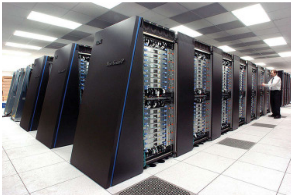
The IBM Blue Gene/P supercomputer at Argonne National Lab runs over 250,000 processors using normal data center air conditioning, grouped in 72 racks/cabinets connected by a high-speed optical network
