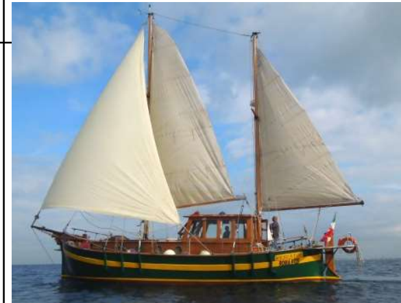
C. Length: 13.20 m, Height: 13 m • Material: wood
